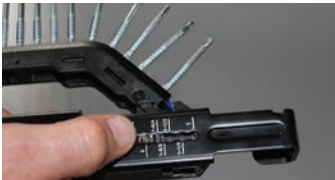
The screw gun is preset from the factory for a 2” (51mm) screw. Confirm that is still set at the 2” (51mm) mark.
