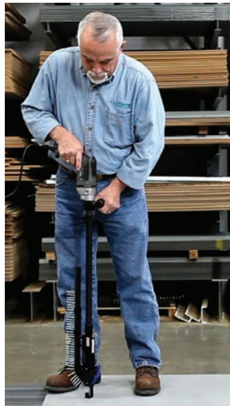
Adjust screw depth by turning the depth adjustment thumb wheel. Refer to the graphics on the tool for proper direction.
