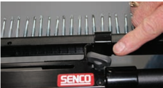
Install the auto-feed end assembly by slipping it over the top of the extension tube and tighten down with the screw adapter until snug.
