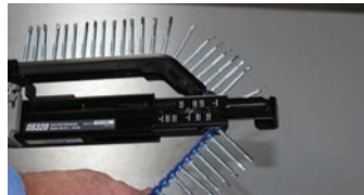
To remove the strip, pull it through the auto-feed end assembly.
