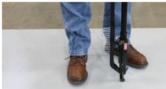
Pull trigger to start motor, press the footplate with constant force against work surface. Do not remove tool from the work until clutch disengages and the bit stops rotating, signaling a fully driven screw. The next screw will be auto fed into place when the tool is removed from the work. This tool has a depth-sensing clutch and will auto disengage making a click ratcheting noise signaling a completed drive.
