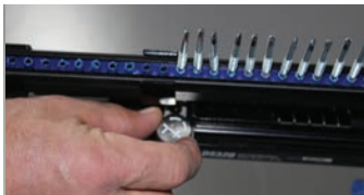
Adjust screw depth by turning the depth adjustment thumb wheel. Refer to the graphics on the tool for proper direction.
