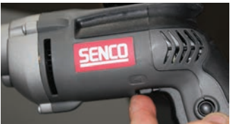
Be sure the screwdriver is operating forward (clockwise) direction. The screw will not advance and bit will be damaged otherwise.
