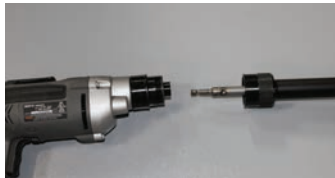
Screw the extension tube onto the screw gun adapter.
