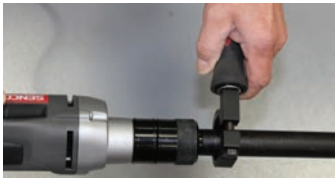
Slip drill handle over extension tube and tighten down.
