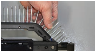
Feed strip into slide body until the 2nd empty slot is aligned with the bit. The tool will feed the first screw when depressed against the work surface.
